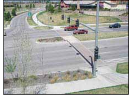
Generous sidewalk widths and a landscaped median to buffer pedestrians from vehicular traffic.
